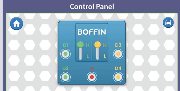
CP has 5 outputs (D1, D2, D3, D4 and A) which are controlled by the app. Outputs D1-D2 and D3-D4 are paired so that each controls a motor in both directions and they can be used to set one of the two levels output voltages, called H (high) and L (low). Output A has a low power output that can control the horn (W1), but cannot control the car's wheel motors. Use the app to control them.
