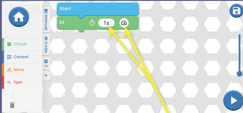
Main field - choose a command from the left menu OUTPUTS/CONTROL/MOVE/TURN and drag it under the command BEGINNING. Command will snap to it. For example D1 from OUTPUTS see picture.
