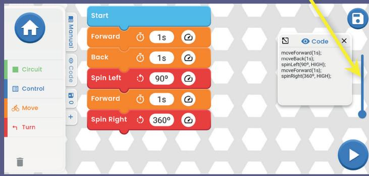
When you enter a command from TURN and click on the 1s time, a window will open where you can set not only the time, but also the degrees of turning (by clicking on Degrees or Time). The degrees are selectable from 0 to 360°.
