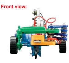
Use the project 34 circuit but add the solar cell (B7) using two 1-snap wires and three 2-snap wires, as shown. Sunlight or incandescent lights can recharge the battery.
