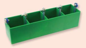
If the copper and zinc electrodes get corroded through use, use sandpaper, steel wool, or a scraper to remove the corrosion and improve performance.
