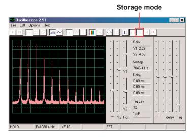
In this way you can show the peak energy achieved at each frequency. But this is only useful on a stable waveform, so if you move the adjustable resistance lever now the signal will fill the screen as the peaks move across the display.
