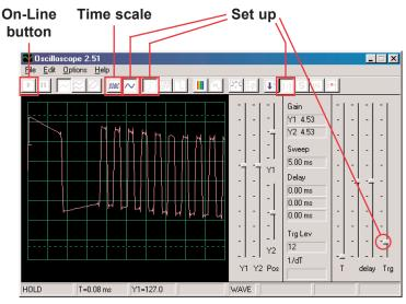
Press the press switch (snap part S2) several times to step through the eight different sounds from the space war integrated circuit. Hold it down for a few seconds each time so you can see the waveform representing the sound you hear.
