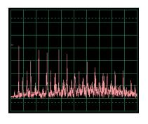
Now put the  $0.02\mu$ F capacitor back in place of the  $0.1\mu$ F capacitor to compare its spectrum. A sample is on the left, with the same Winscope settings as above. As with the oscilloscope mode, its spectrum is weaker and more erratic.
