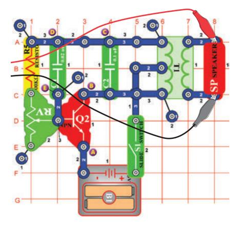
Build the circuit and try the **settings** shown. Move the variable resistor lever to change the pitch of the sound and pulse separation in the waveform.
