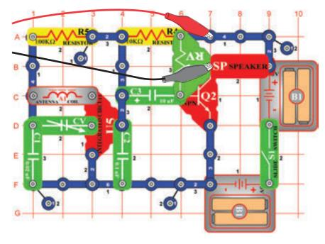
Turn on the switch and adjust the variable capacitor (CV) for a radio station, then adjust the loudness using the variable resistor (RV). Use the same Winscope settings as for project PC12 (AM radio) to view the waveform and frequency spectrum. The waveform will be different from that in projects PC12 and PC38, because those circuits use the power amplifier IC (U4) instead of the PNP transistor for amplification.
