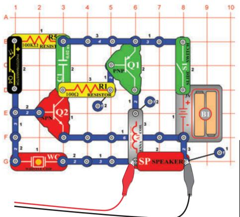
Build the circuit shown. If continuing from the previous experiment then close the Winscope program and run it again, to reset the settings. Set Winscope to the **settings** shown below and click on the On-Line button to activate. A sample waveform is shown here.
