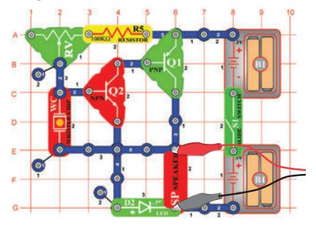
Build the circuit shown, and try the **settings** below. Move the variable resistor lever to change the frequency. A sample waveform is shown here.
