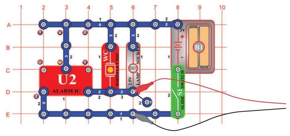
Build the circuit and connect the Winscope PC-interface cable as shown, the cable should still be connected to the microphone input on your computer. If continuing from the previous experiment then close the Winscope program and run it again, to reset the settings. Then use the mouse to **set it up** as shown here, and turn on the switch (snap part S1). Click on the **On-Line button** to activate.
