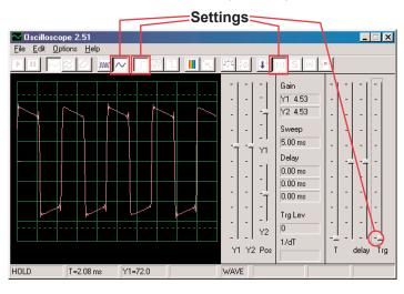
Click on the **5ms/div time scale button** and on the **FFT button** to look at the frequency spectrum for the signal. The Y1 gain control is set for high gain now, so the higher peaks are off the screen but lots of the lower peaks are visible.
