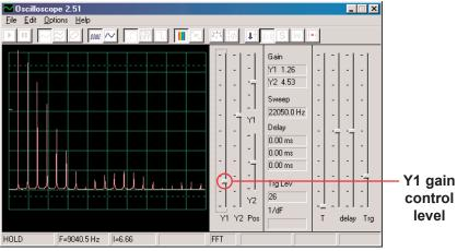
Move the variable resistor control (snap part RV) and watch how it changes the frequencies on the display.
