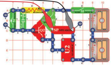
Build the circuit shown. If continuing from the previous experiment then close the Winscope program and run it again, to reset the settings. Set Winscope to the **settings** shown on the right. Click on the On-Line button to activate, turn on the switch, and press the press switch (snap part S2). You hear a siren that slowly fades away.
