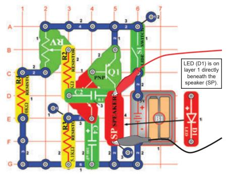
Build the circuit shown. If continuing from the previous experiment then close the Winscope program and run it again, to reset the settings. Click on the On-Line button to activate, and turn on the switch (snap part S1). Set Winscope to the **settings** shown on the upper right, and move the lever on the adjustable resistance (snap part RV) around to change the waveform and the sound. At some positions there may be no sound. A sample waveform is shown on the upper right.
