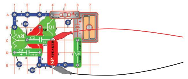
Build the circuit shown. If continuing from the previous experiment then close the Winscope program and run it again, to reset the settings. Click on the **On-Line button** to activate, and turn on the switch (snap part S1). Set Winscope to the settings shown below, and move the lever on the adjustable resistance (snap part RV) around to change **the waveform** and the sound. A sample waveform is shown here, but the pattern and shape of the pulses depends on the adjustable resistance setting.
