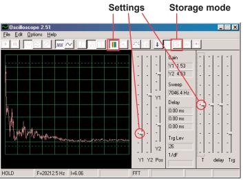
You can also turn on **Storage mode** to see the peaks recorded as you turn the motor, a sample of this is at right.
