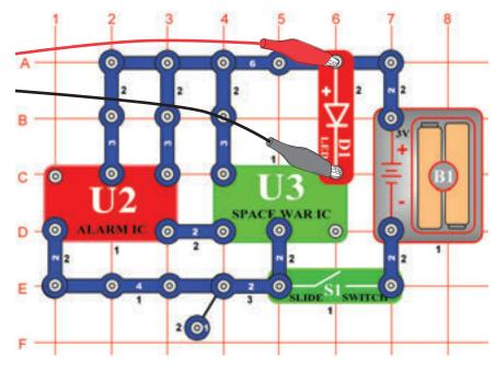
Build the circuit shown. If continuing from the previous experiment then close the Winscope program and run it again, to reset the settings. Click on the **On-Line button** to activate, and turn on the switch (snap part S1). Set Winscope to the **settings** shown below. The signal from the alarm IC (snap part U2) causes the space war IC (part U3) to step through the 8 different patterns it can create. A sample waveform is shown here.
