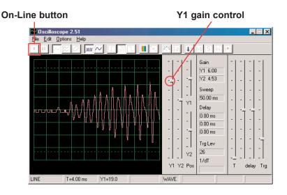
Notice that you need to set the gain control higher here than in the preceding project using the microphone, since speakers were not designed to be used in the same way.
