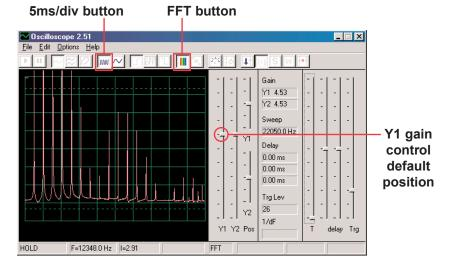
You are seeing the frequency spectrum of your signal, up to 22kHz. Notice that most of the energy is at the low frequencies (below 7kHz), and there is very little as you go higher. The 1:1 gain mode does not apply to the FFT screen, so move the **Y1 gain control** down to here so you can see the peak energy at the low frequencies.
