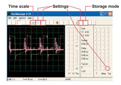
You may replace the  $0.02\mu$ F capacitor C1 with  $0.1\mu$ F capacitor C2 or  $10\mu$ F capacitor C3 to change the sound, but you may want to change the **time scale**.
