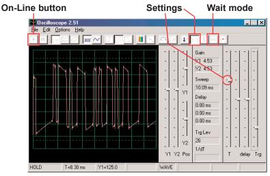
You can also activate **Wait mode** and press the On-Line button several times to view one scan of the signal at a time, instead of seeing continuous scans.
