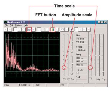
Press the press switch (snap part S2) several times to step through the eight different sounds from the space war integrated circuit. Hold it down for a few seconds each time so you can see the frequency spectrum representing the sound you hear.
