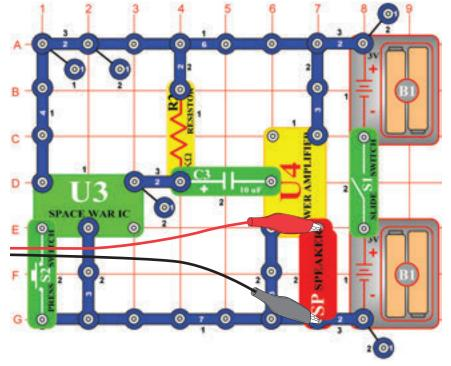
Build the circuit shown and use the same settings as in PC31 to view the waveform. Press the switch (S2) to change the sounds and waveform.
