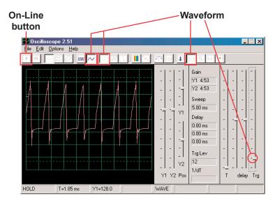
Winscope has a mode that can display multiple scans at the same time, called **Storage mode**. Set the adjustable resistance lever to a low-middle position, place Winscope in this mode, and watch the results.
