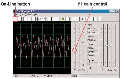
Talk into the microphone (snap part X1) and see what your voice looks like after the microphone converts it to electrical energy. Adjust the **Y1 gain control** to get the best view of it, since the amplitude is greater if you talk louder or are closer to the microphone. Notice how the waveform is different depending on which words or tones you say.
