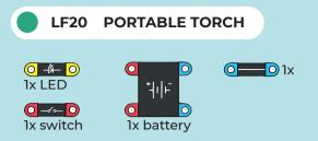
A simple flashlight consisting of a battery, a switch and a LED. When the switch is turned on, the LED lights up and stays on until we turn it off.
