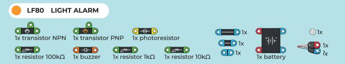
Electronic buzzer, the pitch of which depends on the level of illumination of the photoresistor. A photoresistor with a 1 k $\Omega$  resistor forms a voltage divider whose output voltage is directly proportional to the degree of illumination. The voltage then affects the frequency of the oscillator and thus the pitch.
